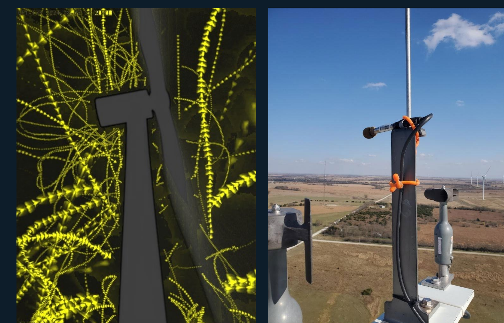
Example composite image showing bat activity captured by thermal cameras. These data were used to develop OSC and estimate exposed bat activity at turbines. Example of an acoustic microphone mounted on the nacelle. These data were used to develop OSC and estimate exposed bat activity at turbines.
